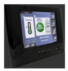
Companion is a control architecture leveraging server-less smart appliances running Linux applications and intuitive Flash interface designs. Capable of managing all aspects of modern home and commercial systems installations using both pre-integrated mode (with inclusive subsystem drivers) and semi-or-full Custom mode control.
