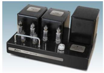
It features a screen voltage regulator and DC restoration circuit minimising crossover distortion and output tube dissipation. 1.5 ohm output impedance and current and voltage feedback loops allow the amplifier to "listen" to the room via acoustic feedback from the speakers.
