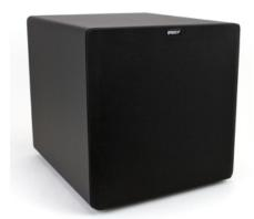
The Energy Power 10 features a 10-inch front-firing woofer, a 50W continuous amplifier, switchable 0-180-degree phase control, rear slot port (increases efficiency), x2 line-level RCA inputs, x2 speaker-level inputs, auto power on and an electronic circuit preventing driver over excursion.
