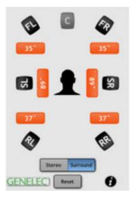
Genelec introduces the SpeakerAngle app for iOS devices, a digital tool which allows anyone to correctly set and match the angling ("toe-in") of both stereo and 7.1 surround sound speakers.
