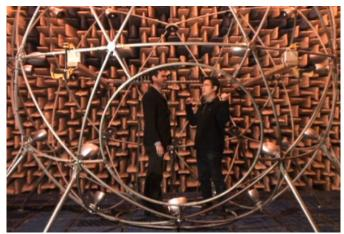
Looking like a spherical cage, the system contains 40 loud speakers set at different positions and allows one to "sculpt" a sonic landscape through the positioning of virtual sound sources within the space.
