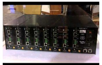
The SmartLink switch is available in 3 versions, each with 8 HDMI inputs and 8 S/PDIF audio-only outputs and a choice of 4, 6 or 8 HDBase T 5Play or HDMI outputs-- in other words enoough control ports for easy audio and video source management.
