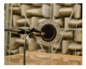
In a part of the world known for its loudspeaker technology as well as its forests, Sweden's KTH Royal Institute of Technology create a new category of loudspeaker with **magnetic cellulose** to generate sound without need of a magnet.
