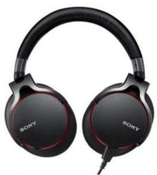
The MDR-27 headphones promise ultra-responsive audio performance with solid aluminium construction, liquid crystal polymer diaphragms and large 70mm drivers. A 4-wire structure separates ground cables to minimise crosstalk between left/right channels and support balanced audio connectors, while silver-coated OFC cable strands reduce signal transmission loss.
