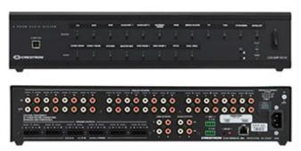
It features 12 inputs, 4 stereo-line outputs, ethernet connectivity and pre-amp controls, and is capable of 100W for each of the 6 amplified zones (with 50W per channel at 8 ohms or 75W per channel at 4 ohms). Installers can also bridge outputs to deliver 150W per channel at 8 ohms to drive an in-wall subwoofer or increased stereo power.
