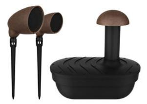
The speakers feature weatherised construction and versatile installation options. Operation is at 8 Ohms with usable frequency range from 80Hz to 20kHz (-10dB), while a built-in transformer allows use with 70 and 100V distributed speaker systems.
