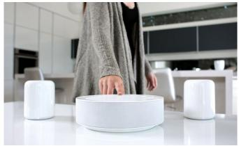
The HiddenHUB features interesting adaptive sound technology making use of an accelerometer to detect whether the speaker is on a flat surface or mounted on a wall. Meanwhile a combination of IR sensors and proprietary logic board scans the room housing the speaker and dynamically adjusts audio to fit the space.
