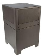
The Omni48AT delivers 360-degree sound from a single location via four coaxially mounted 0.75-inch aluminium dome tweeters over high-excursion 4-inch woofers mated to a crossover network. The 4-inch woofers feature an aluminium cone and Santoprene surround to withstand harsh outdoor environments, and the company says the speakers deliver a balanced musical presentation at any output levels.
