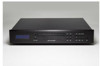
The BCD-3 features a BDA-3 DAC and a fully discrete Bryston Class A analogue output stage with independent analogue and digital power supplies. The transport/laser pickup assembly is partnered with two AKM 4490 384/32-bit DACs, with each DAC synchronised to the transport using a single master clock in order to eliminate jitter.
