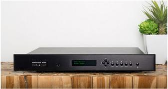
The BDP-3 connects to digital music libraries stored on NAS or USB drives, and streams internet radio and lossless music via Tidal. It carries 8GB RAM, x3 USB 3.0 ports and x2 USB 2.0 ports, with each set of USB sockets sitting on a separate USB bus to improve performance. The USB 3.0 ports make the player compatible with more DAC options, including platforms using the Streamlength protocol.
