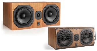
The C3C driver systems feature the ATC SH25-76 dual-suspension tweeter designed and built in-house. The tweeter carries a 15000 gauss (1.5 tesla) neudymium magnet with a black heat-treated top plate, something the company says dissipates heat away from the voice coil to maintain high power handling and low power compression.
