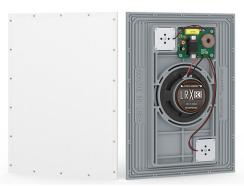
In addition, the LRx83 promises smooth midrange and solid upper frequency for a balanced and high quality invisible speaker. It carries a 30mm midrange device, 25mm tweeter and 8-inch high-power cone woofer, and is able to handle peak power of over 300W. Constant voltage options are also available.
