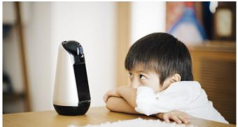
First presented in concept form back at MWC 2016, the Xperia Hello is an Android-based device able to recognise facial expressions and gestures as well as voice through a camera on top of the swivelling "face." The camera is paired with 7 microphones and 4 motion sensors, allowing the Hello to detect people approaching within a 3m radius.
