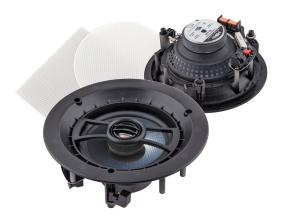
The range includes 5 in-ceiling speakers, all recognisable by an iconic blue cone finish and the use of larger (up to 25mm) pivoting dome tweeters. A recessed woofer and baffle design permits unrestricted airflow to improve low frequency response and more carefully directed high frequency output. Installation promises to be fast and stable through dog-ear fixings allowing installers to work down to 6mm of ceiling thickness.
