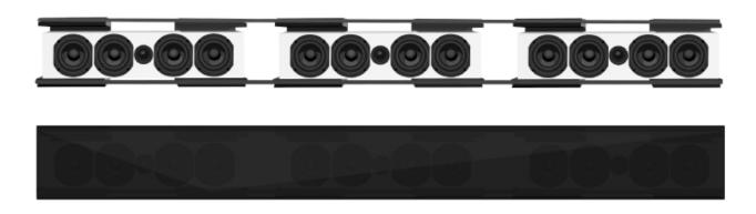
Featuring an 8-ohm impedance, the soundbar incorporates three speaker enclosures with six 3-inch ultra-long throw polypropylene subwoofers with NBR surround sound and a 0.75-inch synthetic soft dome tweeter. It is 9.6cm deep and 15.5cm tall, and is designed for applications demanding a width of 1.4m or longer.
