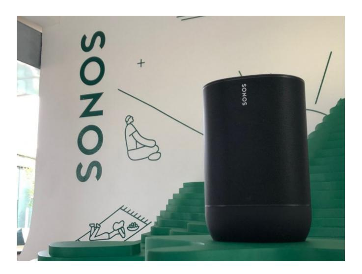
Around 25cm tall and weighing 3kg, the Move promises to be tough enough to handle nearly everything the great outdoors can throw in its direction. The plastic casing is IP65-rated against water and dust, and features a built-in handle. Inside are two Class-D amplifiers pushing a single tweeter and a mid-woofer driver, with TruePlay tuning automatically tweaking the sound to adapt to the environment.
