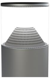
The Big Bollard features a 10-inch burial subwoofer porting out of the sleeve, just before the acoustic lens. Above the lens is a 6.5-inch two-way loudspeaker. Director Collection technology allows the company to keep the width of the sleeve at around 20cm, making it larger than the original model.
