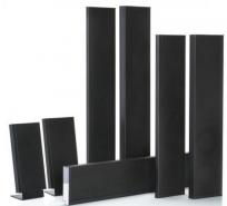
Each Shadow speaker is only 40mm thick and is mountable around or beneath a flat panel TV. Construction is in extruded aluminium, and 4" low profile bass-midrange drivers feature a flat RDT sandwich diaphragm constructed from C-CAM and Rohacell materials, with a unique concertina driver suspension arrangement.
