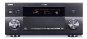
These high-end home theatre receivers introduce new technologies and functions. For example, the RX-V3800 includes 3D CINEMA DSP, latest HDMI 1.3a specification support, upscaling to 1080p, full support for high definition audio formats signals, Adaptive DRC and Adaptive DSP Level, and Network Receiver functions. It features 7-channel surround sound: 980W=140W x 7 RMS; 200W x 7 Max (for Europe).
