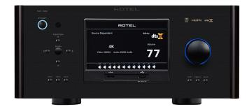
The amplifier section of the RAP-1580 is built on a powerful A/B design, with seven 100W per channel and power from an own toroidal transformer. All channels also use Wolfson 24-bit/192kHz digital-to-analog converters. Inputs include x8 HDMI video inputs (2.0a), with x2 HDMI video outputs supporting 4K video (4:4:4 @ 60Hz 10-bit colour) and x3 inputs and both outputs enabled with HDCP 2.2.
