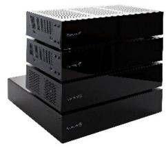
The HDMI switcher is an 8x8 number, and transmits 2D or 3D HD video, multichannel audio, ethernet, RS-232 (serial) and IR signals over a single Cat5e or Cat6 cable via HDBaseT. As well as 8 HDMI inputs and outputs it also features 2 local HDMI outputs, 8 LAN passthrough ports, 8 b-directional stereo audio outputs and a control ethernet port.
