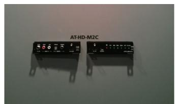
Designed to simplify audio installations, the AT-HD-M2C is converts Dolby and DTS multichannel audio into 2-channel audio, allowing compatibility with legacy devices (such as audio receivers) unable to accept multichannel sources. Built-in EDID provides plug-and-play simplicity, while a variety of output ports (L/R analog, coax, TOSLINK) enable pass-through without HDMI support while retaining audio and video distribution to HDMI displays.
