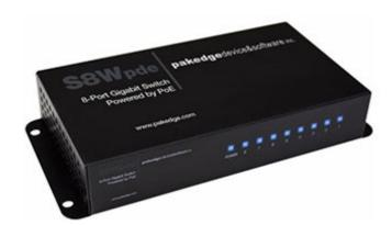
The switch features plug-and-play to run without need for any software installations and is compliant with all network protocols. It takes just a portion of 1U on a wiring rack, and includes a flange-mount bracket for easier installation than traditional cradle-type brackets.
