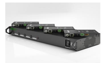
The matrix transmits 2D and 3D video at 60Hz 1080p, with support for 36-bit Deep Colour, HD video and bidirectional control via discrete IR and RS232 over up to 70m of Cat5e/6 cable.
