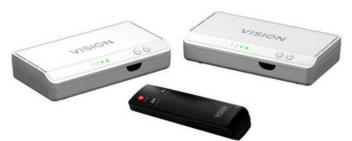
Vision's TechconnectTC2-HDMIP HDMI-Over-Power combines 500Mbps Powerline (or Homeplug) technology with H.264 compression.
