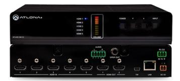
First seen at ISE 2015, the AT-UHD-SW-52ED is part of the SW-5 switcher series. It has 5 inputs and offers 10.2Gbps bandwidth with a web server enabling GUI control over EDID, HDCP and audio settings.
