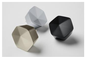
The concept behind the Plume is similar to that behind the <u>Fero router</u> and range extenders. Following initial connection to the ISP's router users simply need to connect multiple pods around the house to create a mesh-like network dubbed "Adaptive Wifi" by the company. The pods work together to ensure the best possible connection and, presumably, provide users with the fastest possible internet.
