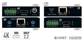
It can also extend signals up to 70m at 1080p/1920x1200 using CAT5e/6 cabling. The extender supports HDR10 at 4K 4:4:4, allowing users to experience a greater range of luminance levels. HDR10 delivery comes as part of the proprietary Full-Buffer Technology (FBT) a system managing TMDS re-clocking and signal regeneration, HDCP authentication to source and display, and EDID handshaking control.
