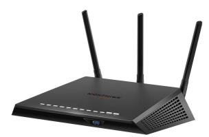
Designed to work with Xbox, PlayStation, Nintendo Switch, PCs and mobile devices, the XR300 tunes the Quality of Service (QoS) towards gaming needs. It offers both wireless and wired connectivity via x3 high-performance external antennas, support for both 2.4 and 5GHz wifi and and x4 ethernet ports, and is powered by a dual-core 1GHz processor.
