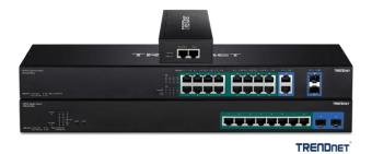
The 4PPoE switches deliver 90W 4PPoE power and networking data over existing ethernet cables. They are unmanaged switches featuring both 4PPoE ports and PoE+ ports. The 4PPoE ports support up to 90W of power per port, while the PoE+ ports support up to 30W per port. Both Gigabit 4PPoE switches include dedicated SFP ports, providing support for long-distance fibre networking.
