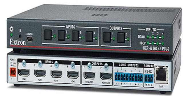
In order to maintain signal integrity and reliability, the switcher provides automatic cable equalisation on each input and independent output reclocking to reshape and restore video signal timing on both HDMI outputs. EDID Minder and Key minder ensure what Extron says is optimal system performance and compliance with HDCP-encrypted content.
