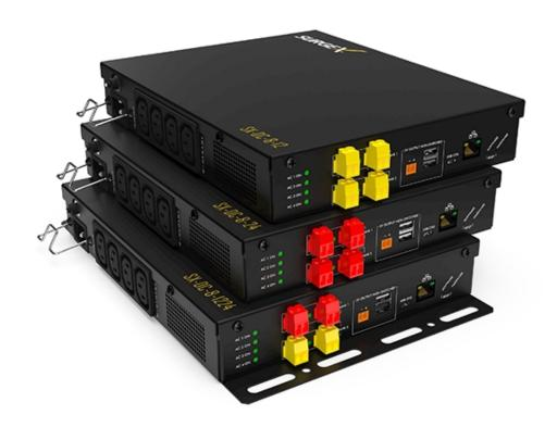
Squid includes two 5V USB ports for charging and network troubleshooting and eight outputs. Four outputs are traditional controlled and monitored IEC receptacles, and four are DC, eliminating the need for wall warts or a two-box solution. Installers can control the AC and DC ports by using a relay-based system, meaning the device can be monitored and easily integrated into 3rd party control systems.
