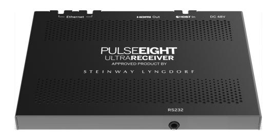
The Ultra Receiver is a HDBaseT 4K60 Type-A compliant receiver solution. It employs DSC technology to enable long-distance transmission (up to 100m) of HDMI 2.0 video (4K 60Hz with 4:4:4 chroma encoding) and 100Mbps ethernet over a single ethernet cable. Just 13mm high, the Ultra Receiver is ideal for discrete installation behind ultra-thin TVs.
