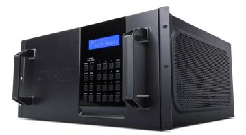
Installers can fit it with any combination of up to 4 input modules and 4 output modules (each with 8 connections per board) for extreme flexibility and performance in any multi-zone AV environments. The company offers a range of input boards, including HDMI, VGA and DVI, while the output board selection includes HDbaseT (100m), HDbaseT (60m with PoC), HDMI and DVI.
