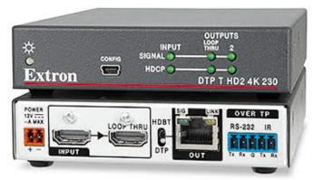
The DTP T HD2 4K 230 extends signals up to 70m, while the DTP T HD2 4K 330 extends signals up to 100m. Both provide x1 HDMI input with loop-through to support local monitoring of digital video and x1 DTP output, with 4K resolution video support including 1080p/60 Deep Colour.
