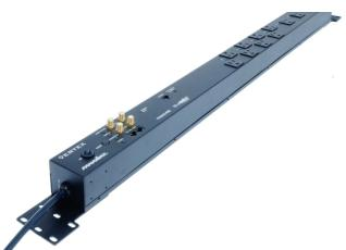
The VT4315 Pro mounts vertically on the back of equipment, and leverages on BlueBOLT IP control technology to control 12 outlets in 8 banks (4 individually controlled outlets and 8 in paired duplex banks). As Panamax puts it, such a configuration enables remote monitoring and reboot in either real-time or via scheduled commands from the connected equipment in the rack.
