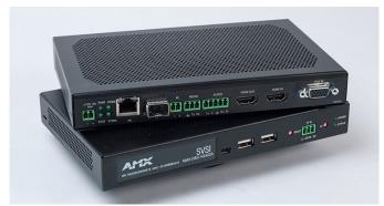
The N2400 series devices support 4K video at 60Hz and 4:4:4 (8-bit colour) through JPEG encoding, and deliver content at native frame rates and colour space with just two frames of latency. HDMI 2.0 and HDCP 2.2 support provides compatibility with all current 4K sources and displays.
