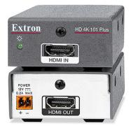
Used at the destination end of a long cable run, the HD 4K 101 Plus actively equalises poor or marginal sources signals, reduces jitter and skew, and adds output pre-emphasis to reliably extended HDMI signals. Extron says it can handle longer distances of up to 22 and 10m for 4K@30Hz and 4K@60Hz signals respectively if paired with an HDMI Pro Series cable.
