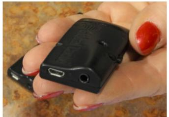
Once connected to a device, the Flex allows for automation with event and task triggers (saved on built-in 4MB flash storage) and web browser access control from network.
