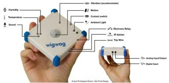
As well as the app the WigWag system contains 3 components-- the Relay, Sensor Block and Glowline. The basic idea involves sensors working with the Relay to trigger user-defined actions, be it sending a tweet or switching lights on or off.
