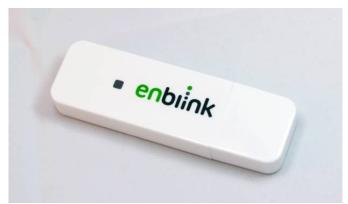
It connects to various devices (such as door locks, lighting systems, IP cameras, sensors) via Z-Wave and provides a control environment on top of the Android-based Google TV interface.
