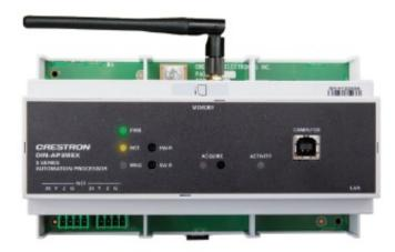
According to Crestron the processors provide an increase in processing power and speed, with modular programming architecture allowing the independent operation and communications of up to 10 programs.
