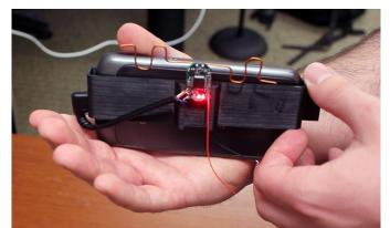
"This is the first gesture recognition system that can be implemented for less than a dollar and doesn't require a battery," UW assistant professor Shyam Gollakota says. "You can leverage TV signals both as a source of power and as a source of gesture recognition."
