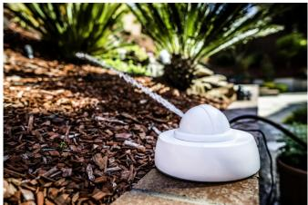
According to the company Droplet lowers sprinkler water consumption by up to 90% via the combination of user configuration and an online plant database. Users set the types of plants to be taken care of via web-based interface, and the sprinkler checks an online database to determine the optimal amount of watering each species requires.
