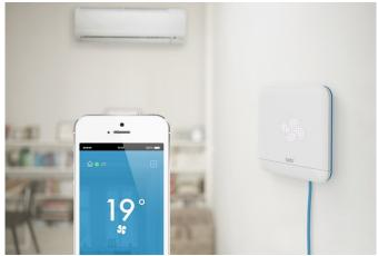
Tado° says Cooling uses geolocation and a Bluetooth LE/iBeacon-based indoor positioning system to monitor home owners, and switches on/off AC units accordingly (for instance it can pre-cool the house when one is coming back from the office). It connects to smartphones via wifi, and replaces the AC's infrared remote to handle control duties.
