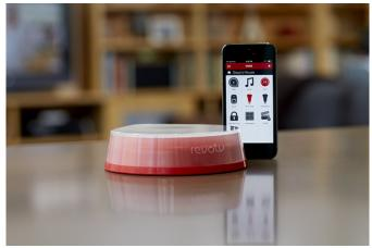
The Revolv product offering consists of a red puck-shaped control device packing 7 radios combined with an iOS app and a cloud-based backend. It handles 10 protocols, and the free cloud service allows the creation of "actions" (aka scenes) based on geolocation, time or sensor activity.
